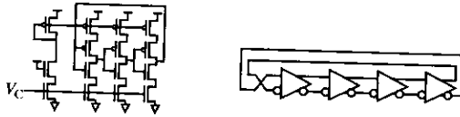
(a) VCO using I-starved inverters (b) VCO using differential delay elements
