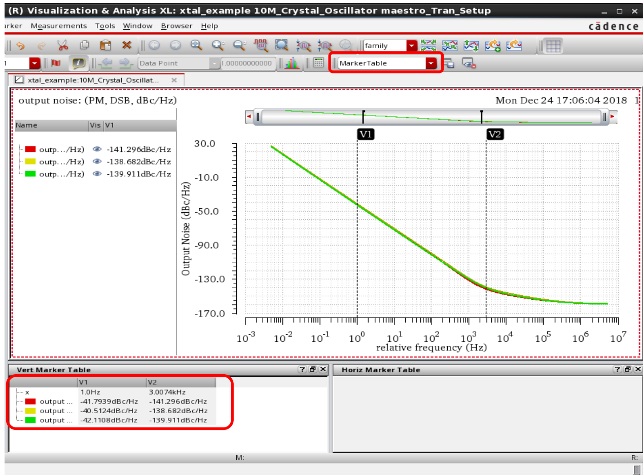
Figure 46 – PM noise plot of Crystal Oscillator – MarkerTable Workspace in ViVA window (when number of harmonics is set to 41 in hb analysis)
